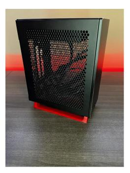
3) Once you have located the mounting position, place the right foot with the brass insert towards the back and thread a M3 x 6mm countersunk screw into the hold and tighten the food down. Leave slightly loose, you will tighten up later.
