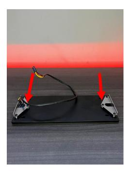
4) Ensure the orientation of the fans when mounting them to the extension. Most fans pull air through the open side of the frame and push out of the grid side. Some fans are different.
