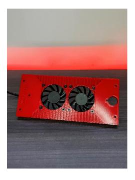
5) Mount the Panel extension to the back of the aluminum front panel with the veins facing the panel and the fan cable to the back.
