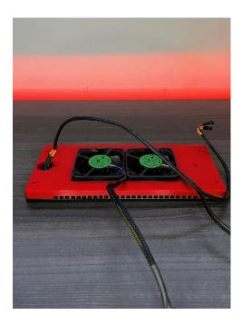
7) Route the front panel power button cables to the motherboard along with the fans to their respective fan headers or splitter. Depending on how your cable management is, you may need to do some additional to allow the fans to clear.
