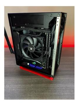
3) Next, take the font panel extension and two 60mm x 10mm fans and screw them into the back of the extension with the provided fan screws. Orientate the cables to the CPU side of the case. **DO NOT OVER TIGHTEN.**
