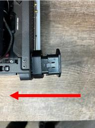
7) Use the provided 6-32 screws to tighten the retention bracket and extension to the chassis. Replace all panels according to the Fractal Design install manual.
