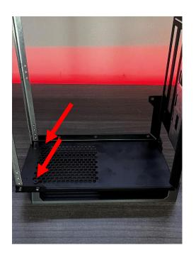
5) Begin re-assembling the side panels at the front of the case first. Before you install the front panel, tighten down the countersunk screws. **DO NOT OVERTIGHTEN.**
