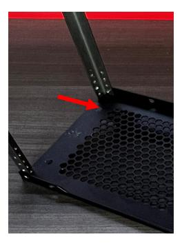
2) With the panels removed, locate the two mounting hex-holes you will be using to mount the front of the case feet to the PSU (top) side of the case.
