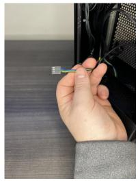
9) Connect your fans to the motherboard and pull any excess cable back through the base. You can then wrap any wire around the fan chassis or zip tie to the integrated cable management loops.
