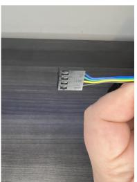
**3)** Looking at the top of the connector with the pin retention access, use your pin or pick tool to push down on the tabs to release the pins from the connector. Note: you will not need to use much for to release the tabs. Do one wire at a time.
