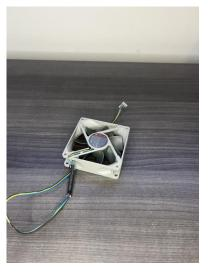
**2)** Take a picture or write down the orientation or the wires in the connector, as you will need to remove the pins in order to install into the case.
