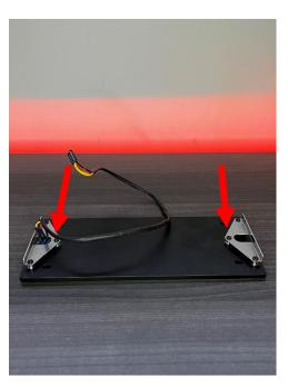
4) Next, attach the front panel mounting brackets using the included six M3 x 20mm button head screws. DO **NOT OVER TIGHTEN!**
