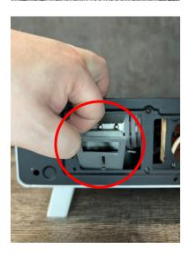
4) Slide the assembly over until it lines up with the two mounting holes.
