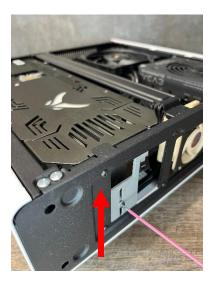
7) Failure to leave at least 5mm of clearance may case the case panel to not close properly or scratch your GPU. Replace the top panel and front IO panel per the Ridge install manual.
