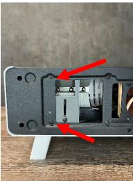
6) With the bracket fastened to the chassis, slide the adjustment screw up to meant the GPU and continue until there is roughly 5mm of clearance between the GPU and chassis mounting tap. (See figure 7)
