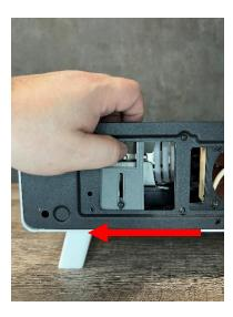
5) Insert the 3mm screws into the assemble and tighten with a 2.5mm Allen wrench.
