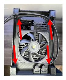
5) Route your fan cables and/or USB cables down through your case and to the Motherboard. Reapply you rubber feet onto the new base.
