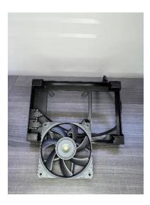
4) Once you have your fan and/or USB mounted place the base on the bottom of the case with the cutout to the back and the fan to the front of the case. Use the SSUPD provided 6-32 "feet" screws to mount the base to the bottom of the chassis.
